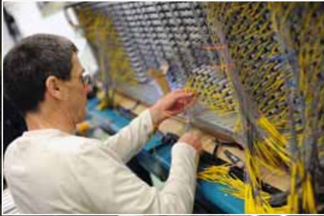
Constructing an electromagnetic calorimeter at Lancaster for the T2K neutrino experiment in Japan.
