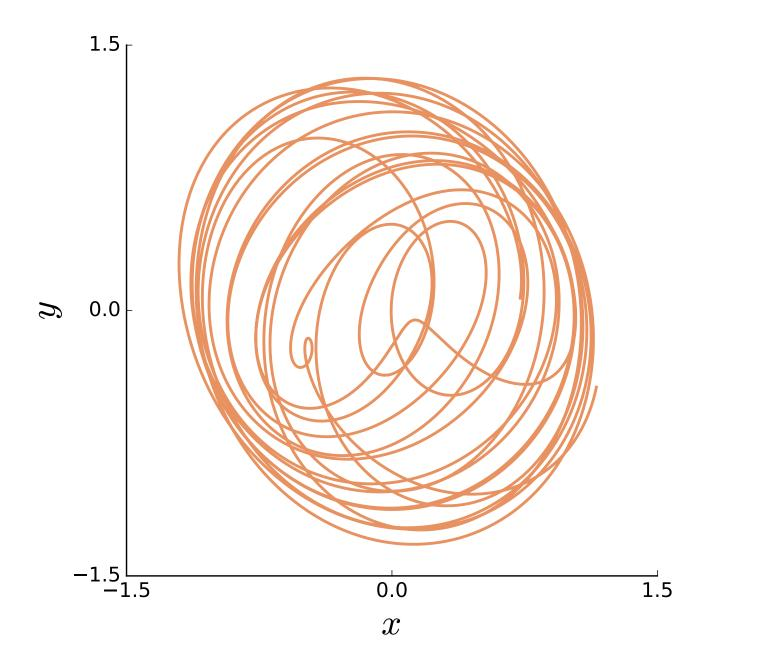
Fig. 1: Forced Poincaré oscillator. One trajectory in state space: no clear attractor.
